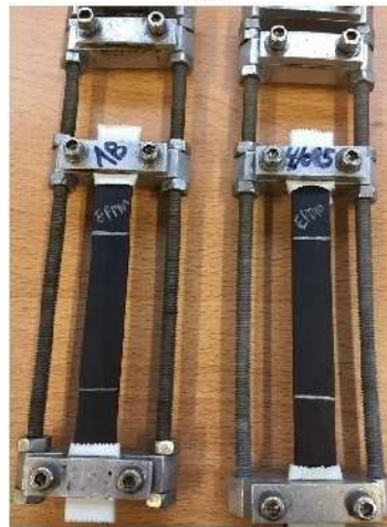
Photograph sample EPDM after oxone resistance test.
