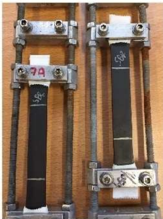
Photograph sample SRR after oxone resistance test.
